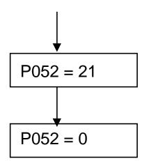
With DC BUS connected to the COMMON DC BUS of the system, set P52=21 and provide a start command at terminal X101, pin #9
